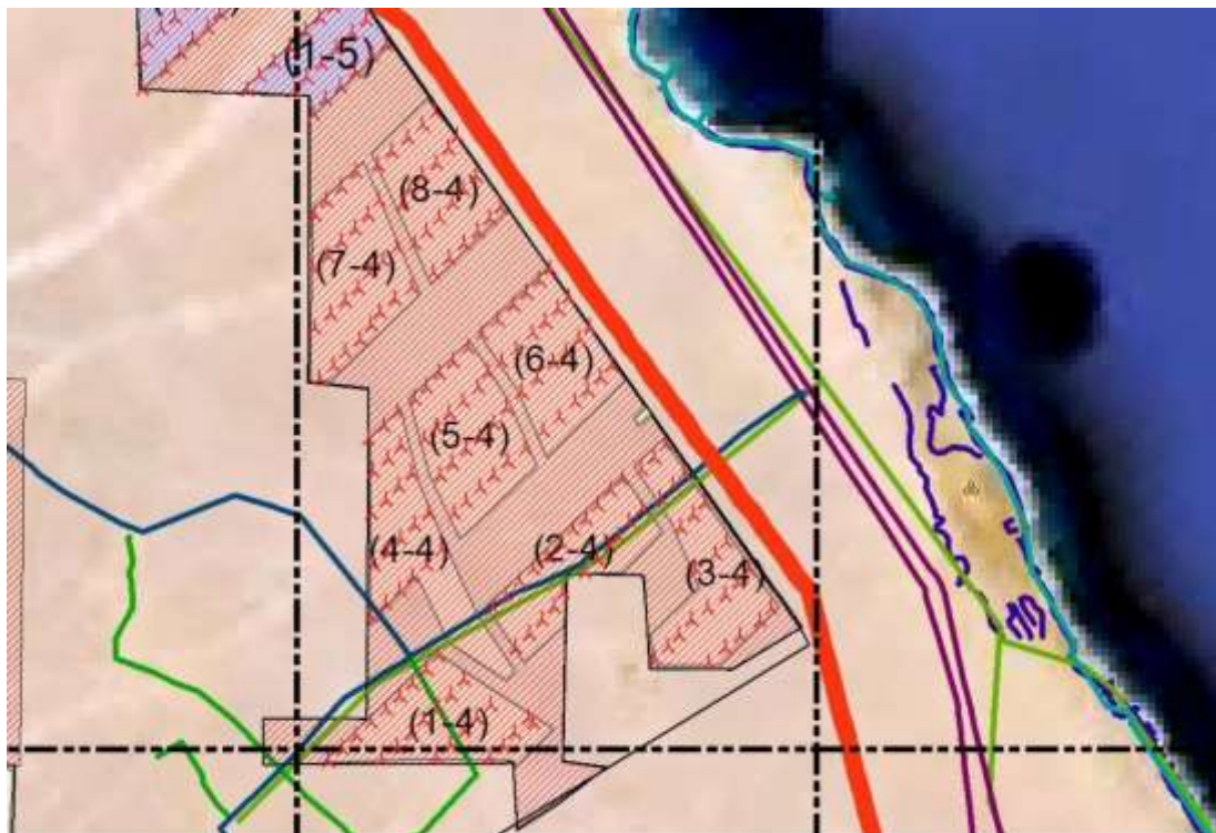
Figure 1.5: Example of a typical arrangement of turbines in rows in the southern part of the 284 km 2 project area (taking into consideration the provided Wind project-plots)
