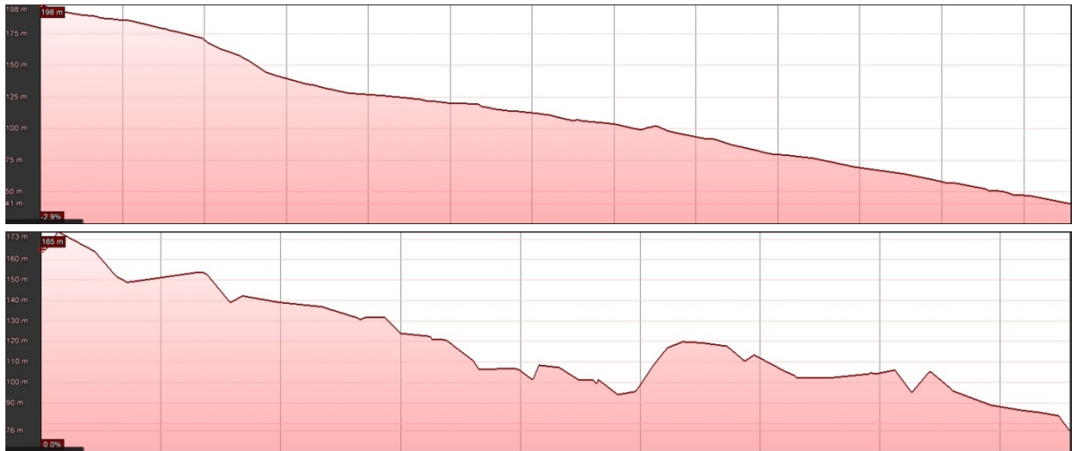
Figure 1.1: Topographical profiles of the project area (top: cross section through the southern part of the project area from south-west (left) to north-east (right); bottom: lengthwise cross section through the project area from north-west (left) to south-east (right) (route of sections can be taken from the Google Earth-image at the top))
